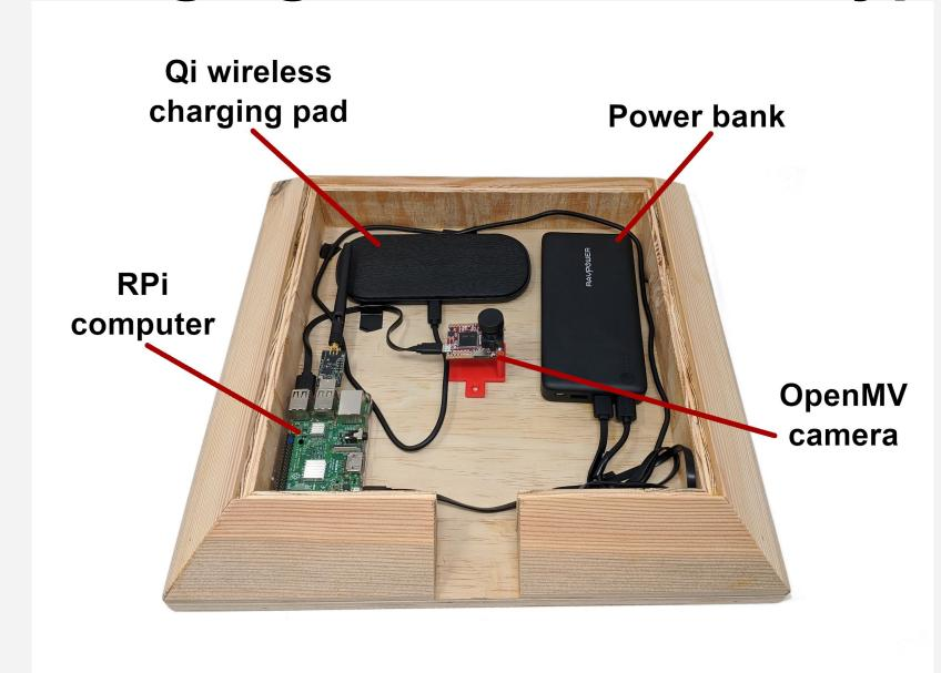
The modular nature of the charging platform allows for reconfiguration to fit the specified requirements of any particular deployment. 3D printed mounts with screw tabs have been created to allow for all components to be firmly stationary while still allowing changes. Software on the platform is also built to object-oriented standards to allow substitution of the UAV. As we intended this platform to be low-cost, all software and schematics are freely available under open-source licenses.
