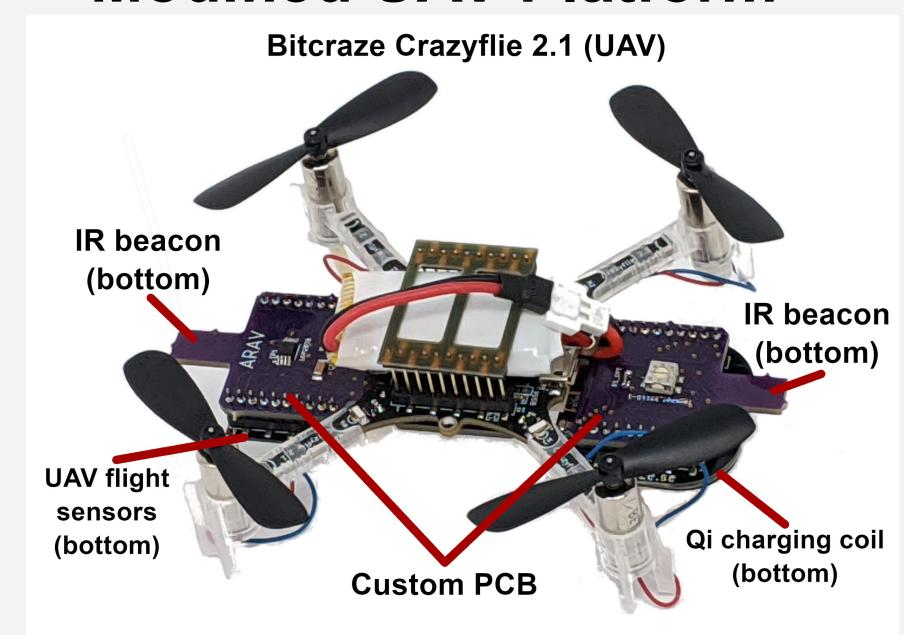
UAV modifications allowed for better tracking via IR beacons as well as an increase in the functionality of the UAV platform. Due to the increased weight of the custom PCB, new motors were added which, combined with the IR beacon circuit, increased power consumption and reduced potential flight time. The custom PCB is also necessary to support simultaneous mounting of the flight sensors and Qi charging coil on the UAV.
